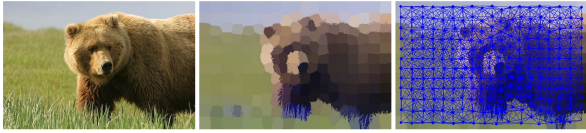
Figure 2: Illustration of the process to transform an image into the graph. First column, second column and third column show original images, superpixels obtained by SLIC and the resultant graph.
