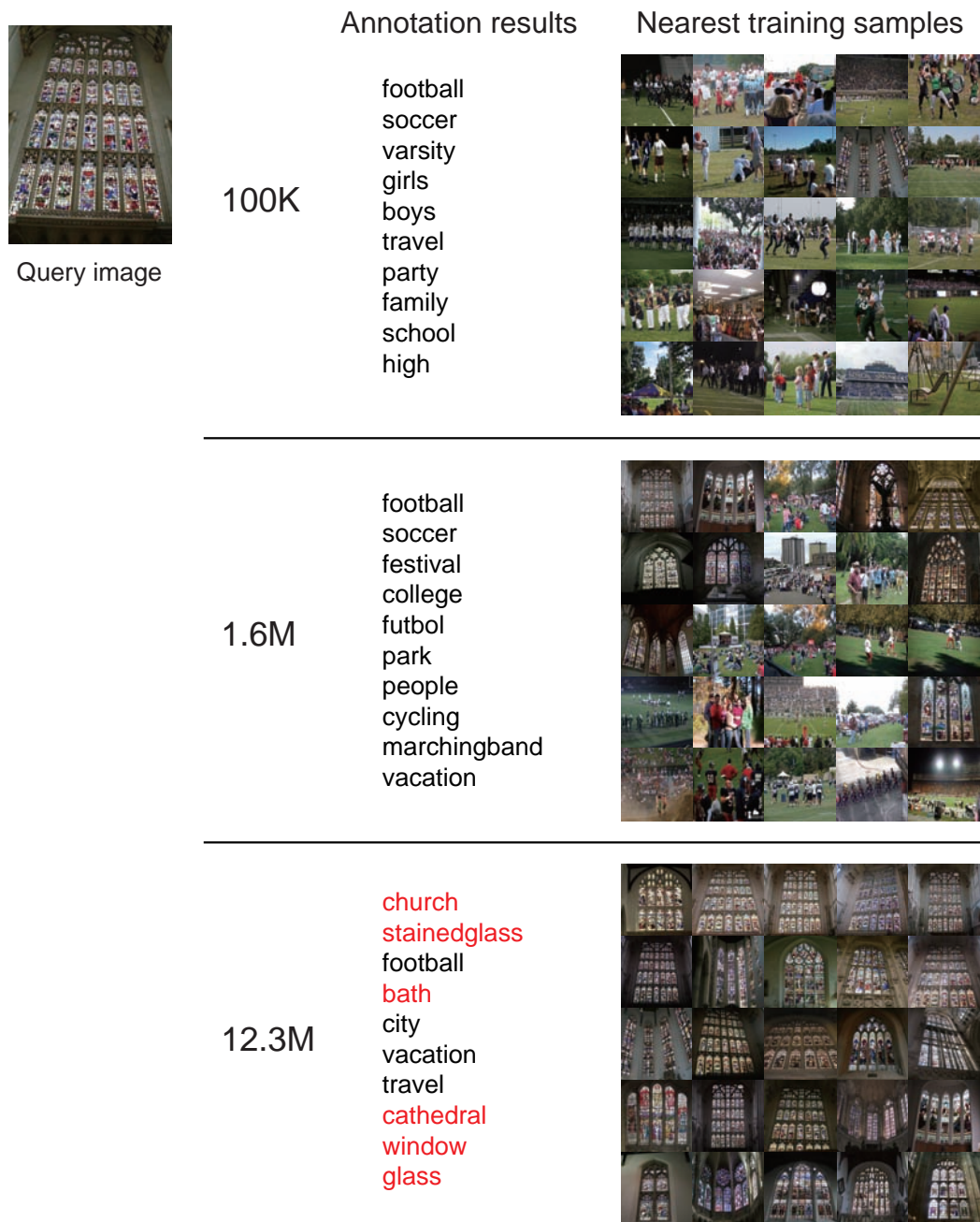
Figure 7.8: (1/3) Example of annotation using a varying number of training samples. Correct annotations are written in red. For each case, the 25 nearest images are shown.
